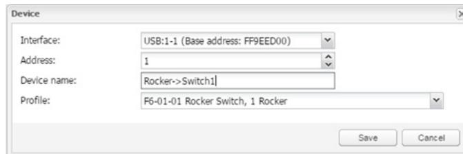
Once the device is added, pair it with specific device in EnOcean network. Set the EnOcean device in learning mode and then press Teach-in button in spaceLYnk configuration.
