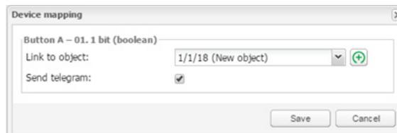
When KNX object value is changed (1/1/18 in the example above), telegram is sent to the device, which has been paired with spaceLYnk virtual device (F6-01-01 in the example above).
